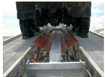
C. The undercarriage washdown unit provides 90% of the cleaning task. Twelve nozzles spray 40 gpm. This unit travels up and down the central canal at the operators command with a push button system.
