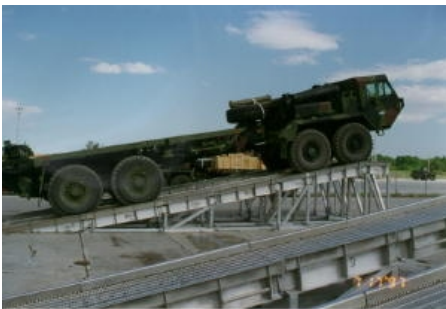
A. CAWF is integrated with VSR3635 service ramps. Pictured is a LVS in position for cleaning.
