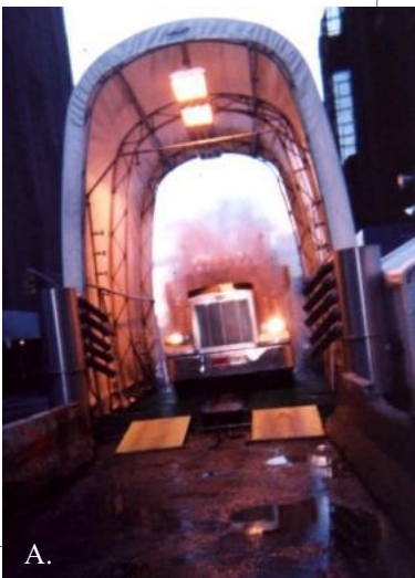
A. Heavy vehicles slowly enter the system and are sprayed by a series of multi-direction high pressure nozzles that remove truck and debris contaminants.
